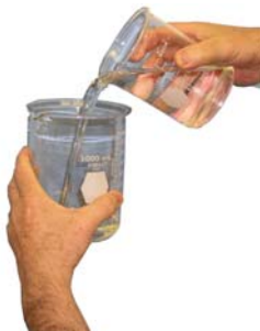
PSF-0.65cSt HMDS is a Hexamethyldisiloxane fluid with the lowest viscosity and lowest surface tension of the PDMS Silicone Fluids
