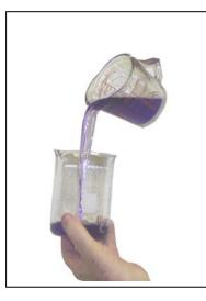
DOT 5 Silicone Brake Fluid is a hydrophobic fluid that provides excellent lubrication and corrosion protection. **DOT 5 Silicone Brake Fluid (DOT V)** is formulated for use in hydraulic brake systems at ambient temperatures ranging from  $-55^{\circ}$ C to 55°C. It has a bluish-purplish viscous fluid. DOT 5 Silicone Brake Fluid is identified by military symbol BFS and NATO code No. H-547 and meets Mil –PRF-46176.
