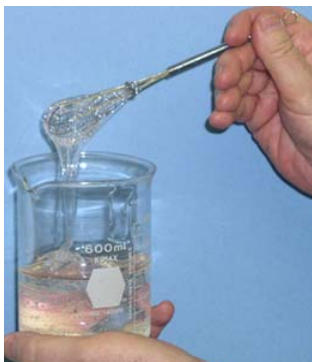
Super Hi-Viscosity Silicones Fluids are extremely viscous PDMS Silicones that meet VV-D-1078 "Silicone as Damping Fluid" and are used in a wide range of damping applications.
