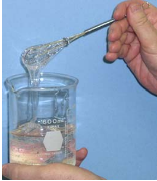
Clearco Super Hi-Viscosity Silicones Fluids are extremely viscous fluids that meet VV-D-1078 "Silicone as Damping Fluid" and are used in a wide range of damping applications.
