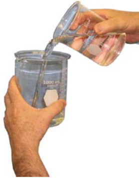
Pure Silicone Fluid 1cSt has a viscosity of water.
