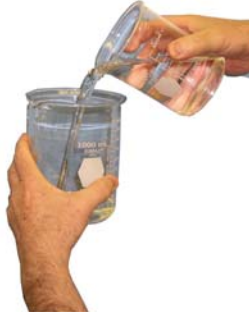
Pure Silicone Fluid 20cSt is a low viscosity 100% silicone with a viscosity slightly higher than water.
