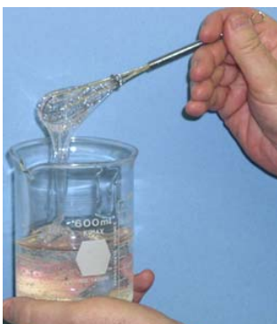
Pure Silicone 12,500cSt is a high viscosity silicone with a consistency of honey.
