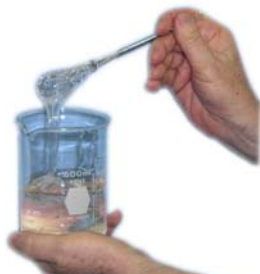
PSF- 30k & 60k are high viscosity PDMS Silicones that meet federal spec VV-D-1078 "Silicone as Damping Fluid".
