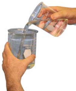
Pure Silicone Fluid 1.5cSt has a viscosity similar to water.
